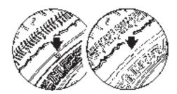
Continental Tire has introduced an innovative new system of preventative maintenance aimed at protecting the sidewall. The Sidewall Rib Guard with curb scuff indicators allows the customer to monitor the abrasive affects of repeated curb/sidewall scuffing and takes the guesswork out of determining the remaining thickness of a sidewall after frequent scuffing occurs.
